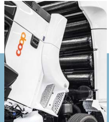
High-pressure storage unit for truck
