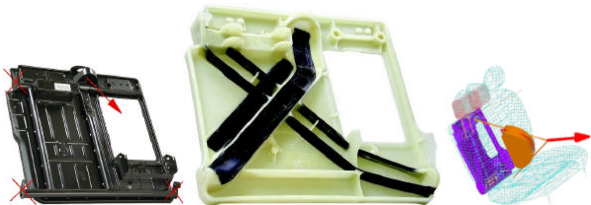
Figure 5: (left) metal seatback, (middle) E-LFT seatback, (right) middle seatbelt joint
