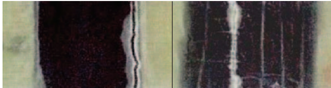
Fig.11: critical and subcritical crack-propagation by dynamic loads.
