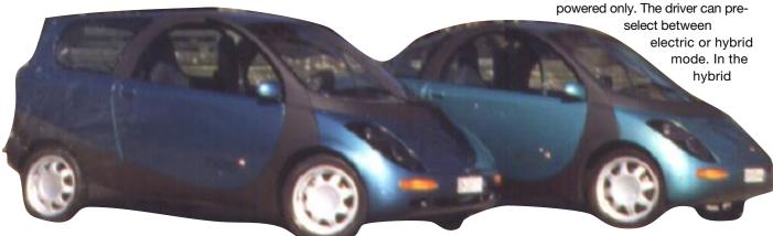
mode, a downsized, two-cylinder, four-stroke aluminium engine will add power to the motor for speeds above 60km/h.
